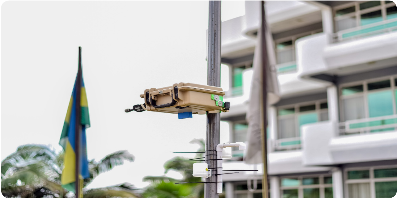
One of the sensors (installed at AIMS Headquarters) which will support in monitoring noise and air pollution
