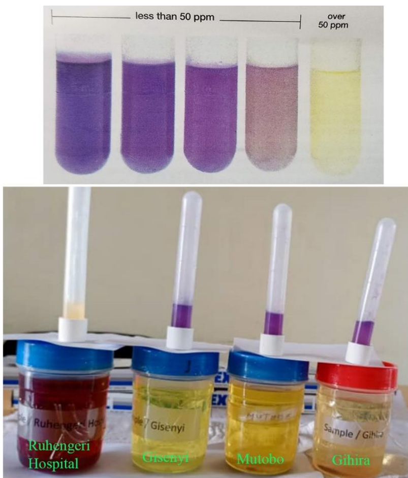
Figure 3. 5: PCB determination in oils which are in service (the above part of the figure is the reference from the manufacturer of the test kits).
