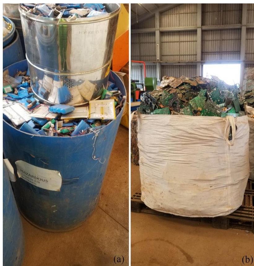
Figure 6. 13: E-wastes resulting from dismantled EEE waiting to be sent abroad for recycling: (a) Lithium-ion batteries; and (b) Motherboards.
