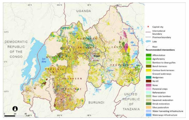
Figure 5-5: Recommended interventions for erosion control in Rwanda (Source: RWBA, 2021)
