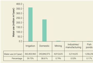
Figure 6-5: Consumptive water uses by sectors during 2019 (RWB, 2021a).
