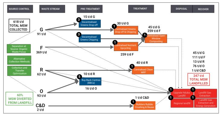
Figure 7-11: MSW Flow proposed for Kigali City (Vice, Rugege, & Benitez, 2019). Note: The waste stream options formulation was based on different waste minimization categories 0: supply chain, 2: Reuse, 3: Recycling, 4: Recovery, 5: Disposal. Greens (G), Food Waste (F), Recyclables (R), Other Waste (O) and Construction and Demolition Waste (C&D).
