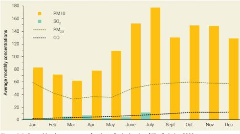
**Figure 8-2:** Ground-level measurement for air quality in the city of Kigali, during 2020 Note: Data was not available for August. SO<sub>2</sub> measurements were only available for January-July. The units of measurements for PM <sub>2.5</sub> and PM<sub>10</sub> are  $\mu$ g/m<sup>3</sup> and CO is ppm. Data Source: REMA, data from Kigali reference station 2020
