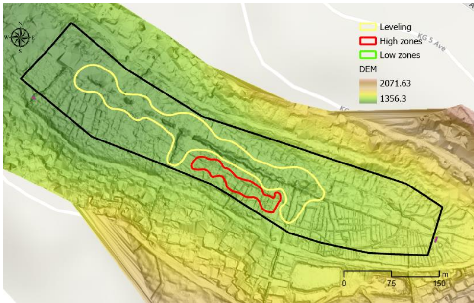
FIGURE 5-62: SOIL RESHAPING FOR WETLAND CREATION – RU15A
