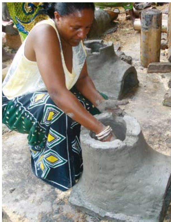
Energy saving cook stoves like these being made can reduce the amount of fuel wood that is used for cooking purposes
